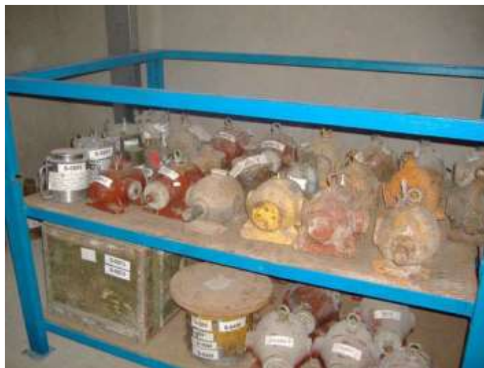
Fig. 8: Disused sealed radioactive sources in the interim storage.
