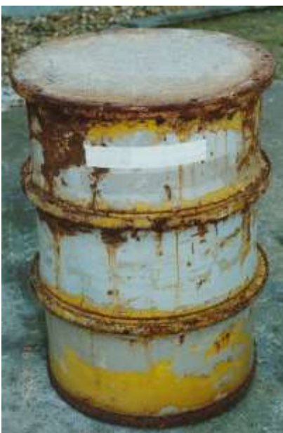
Fig. 1. Corroded drum with cemented radioactive waste after several years of interim storage.
